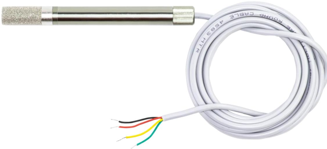
This sensor is a high-precision industrial-grade RS485 temperature and humidity measurement device utilizing the advanced sensor. Designed for robustness, reliability, and accurate digital signal processing, it converts ambient temperature and humidity into reliable RS485 signals for seamless integration with centralized monitoring systems.
